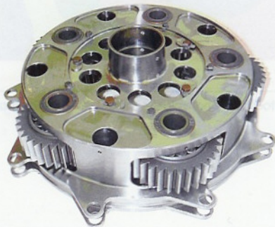
Figure 9—Second-stage carrier assembly.
