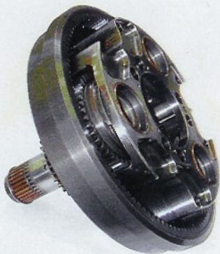
Figure 7—First-stage carrier and ring gear assembly.
