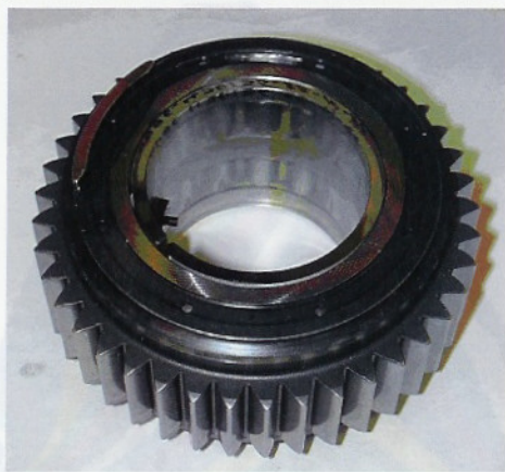
Figure 8—Second-stage sun gear.
